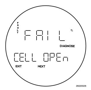
Figure 6-9. Fault 5, O<sub>2</sub> Cell Open
